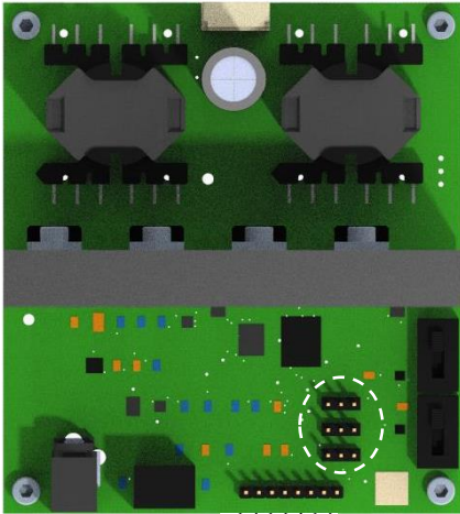
ECU pins identification
